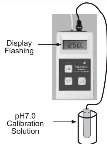
Figure 6. Typical Calibration Display
