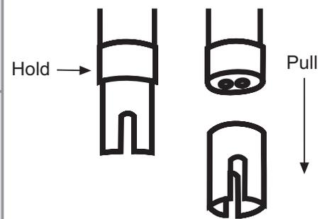
Figure 5. Shroud Removed
